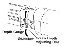
①Turn the screw depth adjusting dial upward to achieve more depth.
